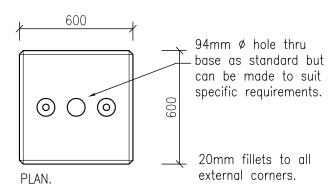
2No semi—spherical recess in gravitational centreline of block for pin anchors. (pin anchor is rated at 2.5 tonnes with a F.O.S. of 3)
